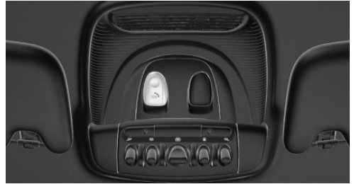
SOS button in the roofliner
